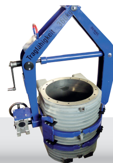
90° (centre) and 360° (right) rotating clamps with spindle adjustment and self-locking drive
